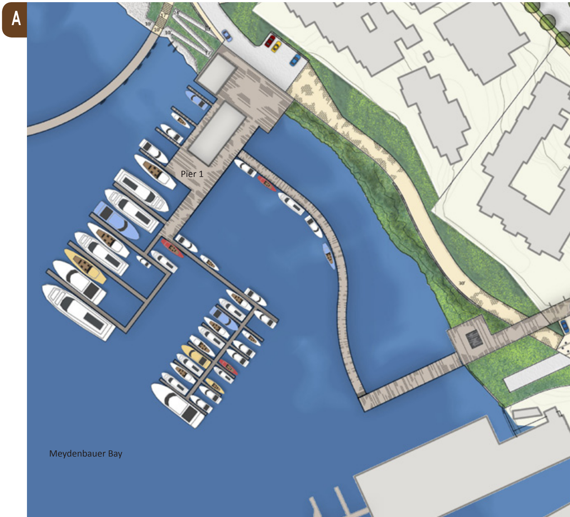
A Figure 2.5-7: Reconfigured Marina - Expanded Pier 1
